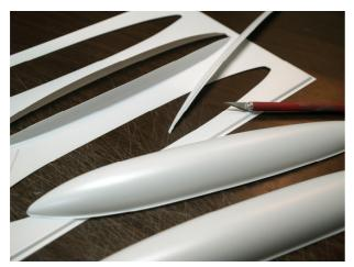
To begin assembly cut the tank doublers from the center of the parts sheet. Separate the doublers by cutting them along the bottom of the 'V' groove. This will form a stiffener along the sides allowing you to apply clamp pressure later. Only about ¾ inch at the center, tapered to a blunt point at the ends of the doublers is needed.
